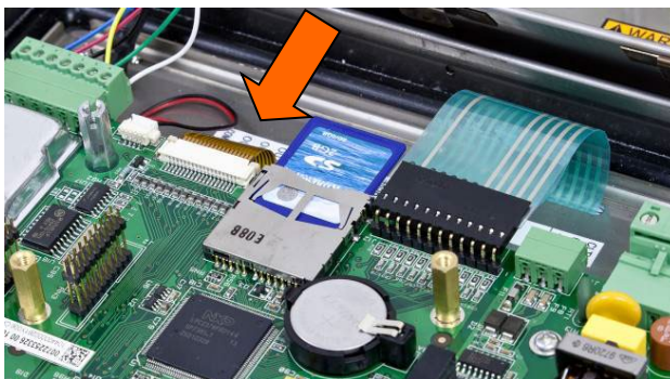
Figure 5-14: Insertion de la carte Mémoire SD
